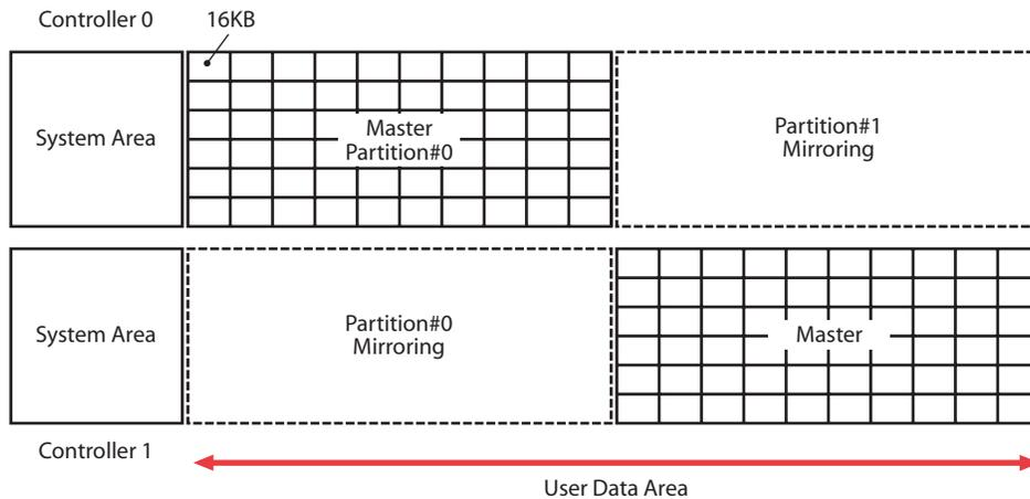
*When the Cache Partition Manager feature is employed, each side of the cache is allocated to a controller and assigned a master partition.*
