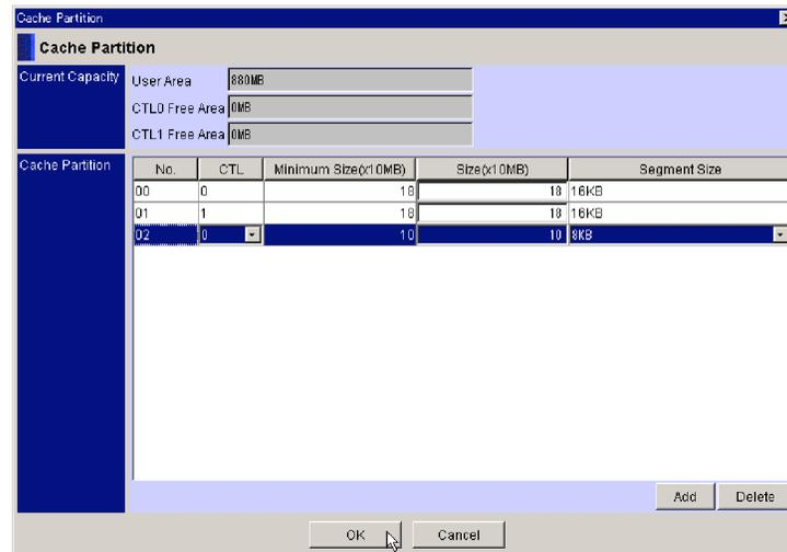
Once a cache partition is created using the Cache Partition Dialog Box, it must be assigned to an LU in the storage system and the system must be restarted for changes to take effect.
