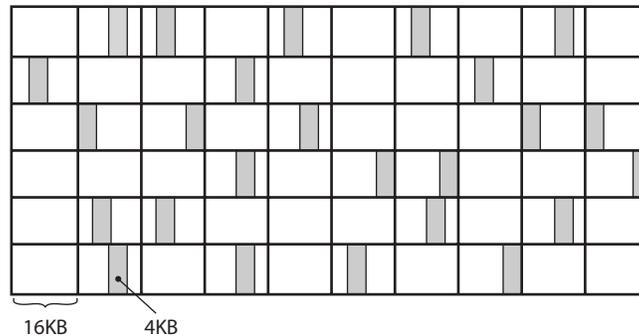
*The inefficient use of the cache—smaller I/O from an application placed in a larger system-allocated cache segment—can contribute to poor cache hit ratios, causing the storage system to replenish cache from disk more frequently.*
