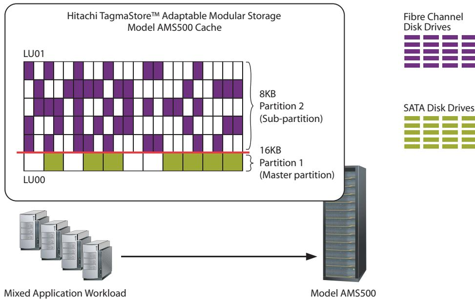
*The Cache Partition Manager feature allows the cache of the Adaptable Modular Storage system to be allocated to disk drives that are likely to make the best use of the resources.*
