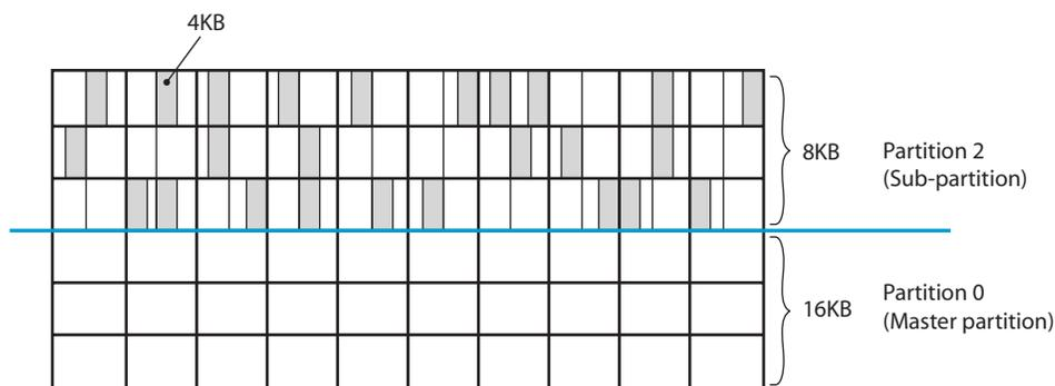
*The Cache Partition Manager feature allows the cache resources of the Adaptable Modular Storage and Workgroup Modular Storage systems to be divided into multiple partitions, which can be allocated a different segment size.*
