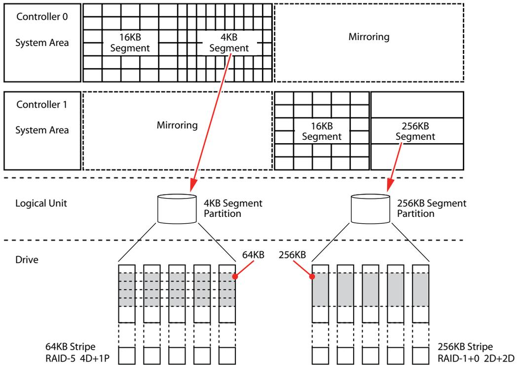
*Changing the cache partition segment size to match the LU strip size allows data to be sent or received to or from a disk drive more efficiently.*
