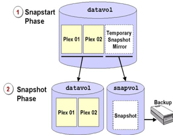
Figure 2: FlashSnap creates, detaches, and resynchronizes a snapshot mirror of an original volume.
