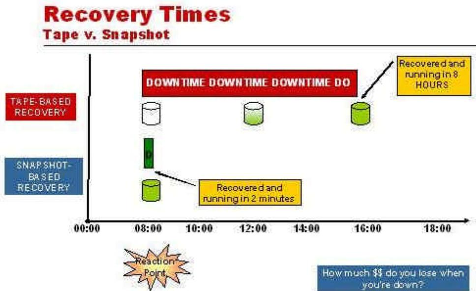
Figure 1: Restoring from a snapshot eliminates the time spent restoring from tape, speeding recoveries significantly.
